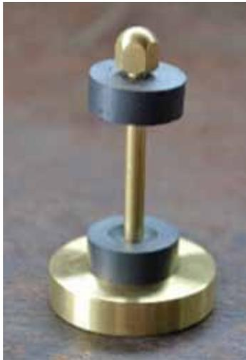
The first one has magnets in vertical opposition, with a lower magnet resting on its brass base. The magnet above is pushed 1.125" higher by opposing flux, complete with its 10 gram weight. Space between the magnet faces remains constant under normal conditions.
