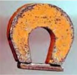
Early 'Eclipse' horse shoe magnets for general use came with a keeper placed across the poles to prevent loss of magnetism. The keeper being removed to expose the magnets ready for work. A horse shoe magnet is made of alnico, an iron alloy. The magnet, made in the shape of a horseshoe, has the two magnetic poles close together. This shape creates a strong magnetic field between the poles, allowing the magnet to pick up a heavy piece of iron.
