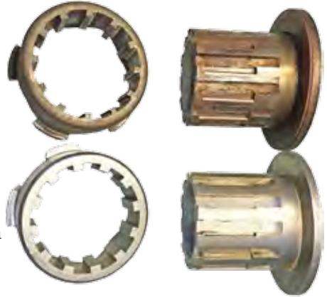
By the way, I haven't seen any of the later shock absorbers with worn out splines, yet. Probably the oil from the engine reaches this better. A few ones have had chewed up ramps, though. This is certainly caused by the ramps 'going over the top'. They should never be able to do that, so further investigation is needed before fitting new parts, if this has happened.
