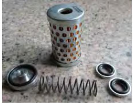
The filter element is a high quality, standard proprietary item originally designed for modern Royal Enfield engines and replacements are available from local Royal Enfield dealers, as well as from Criterion. Pattern filters are also available very cheaply on eBay, but these are often of poor quality.
