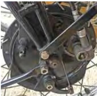
a disappointing brake and I frequently reverted to a single leading shoe brake which was better. When the custom linings for the TLS brake were returned the linings were twice the thickness they had ever been, problem cured, the brake is now excellent. Personally, I'm wary of riveted linings as it probably means they are off the shelf and old, modern bonded linings machined to fit optimises the available braking capability.
